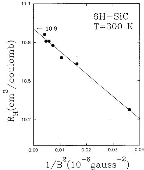
FIG. 1. The plot of Hall coefficient  $R_H$  vs  $1/B^2$ . The solid line is a linear plot, which has been extrapolated to  $B \rightarrow \infty$ .
