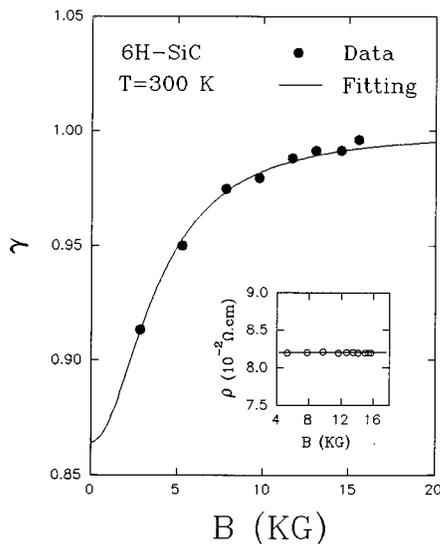
FIG. 2. Hall factor  $\gamma$  of 6H-SiC as a function of the magnetic field measured at room temperature. The solid line is a least squares fit by Eq. (3). The inset is the plot of the sample resistivity as a function of the magnetic field.
