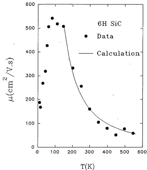
FIG. 3. Electron mobility  $\mu$  as a function of temperature for a nitrogen doped 6H-SiC sample. The solid dots are the experimental data and the solid curve above 150 K is the calculation result using  $\mu = A'T^{-1.67}$  with  $A' = 2.2 \times 10^6$ .
