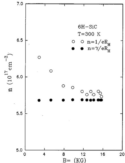
FIG. 4. The electron concentration  $n$  as a function of the magnetic field with (●) and without (○) the correction of the magnetic field dependence of the Hall factor  $\gamma$ .
